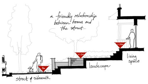
Figure 10: Relationship of residential entries to public sidewalks and walkways in elevation.
