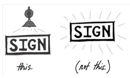
Figure 13: Backlit signs should be avoided in favour or raised or recessed letters that may be externally lit.
