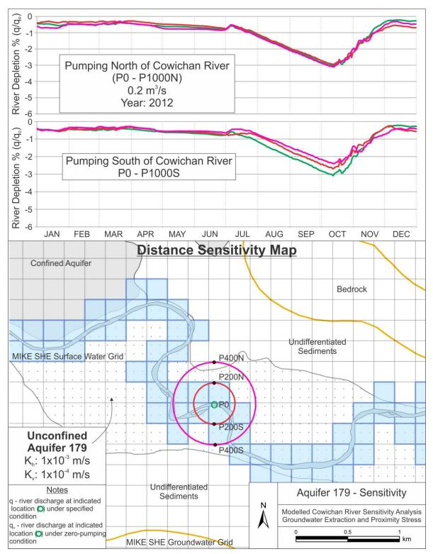
Figure A2.1. Modelled Cowichan River distance - sensitivity assessment for Aquifer 179 (0.2 m<sup>3</sup>/s pumping rate).
