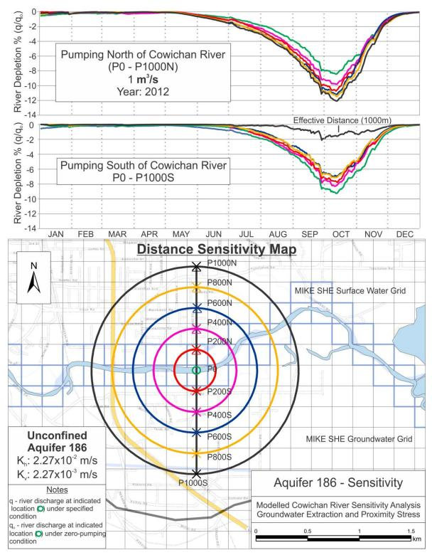
Figure 3.20. Modelled Cowichan River distance - sensitivity assessment for Aquifer 186 (1 m<sup>3</sup>/s pumping rate).
