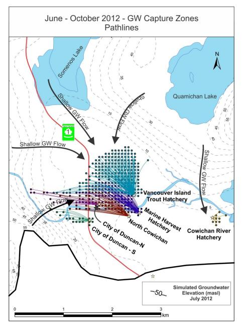
Figure 3.13. Summer low flow season transient capture zone analysis results for the major GW extraction users within the lower valley. Shown are the particle pathlines within the shallow aquifer materials.
