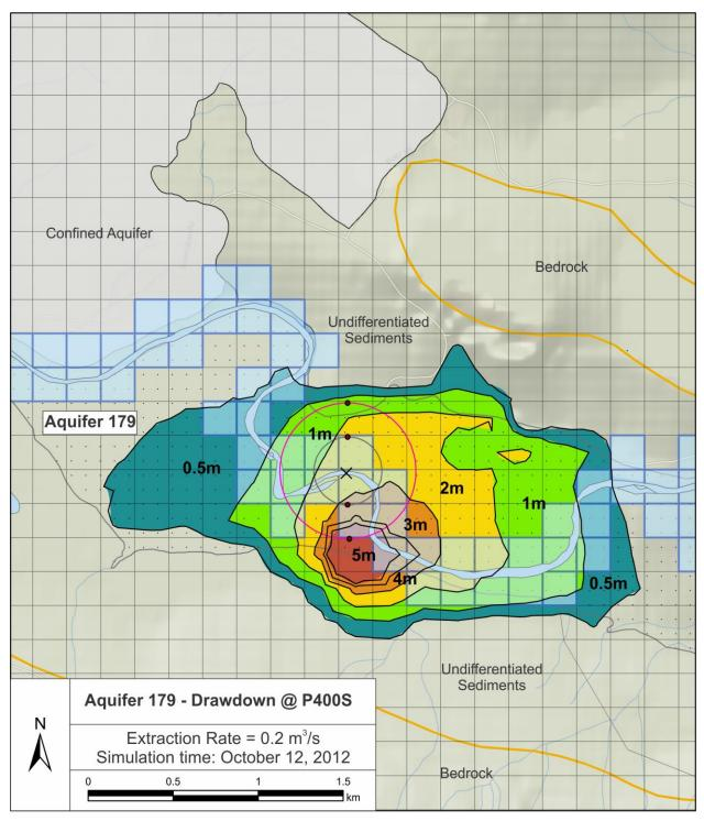
Figure A2.3. Drawdown during distance - sensitivity test. Pumping occurring at P400S location (0.2 m<sup>3</sup>/s).
