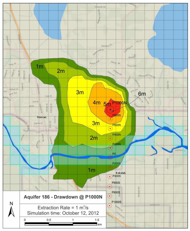
Figure 3.22. Drawdown during distance - sensitivity test. Pumping occurring at P1000N location (1 m<sup>3</sup>/s).
