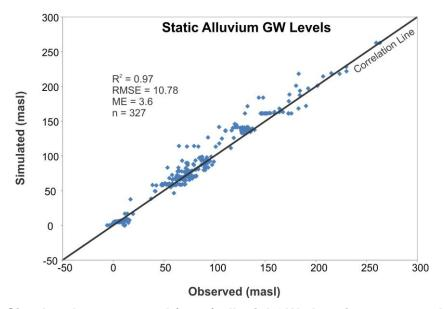
Figure 3.1. Simulated mean annual (2007) alluvial GW elevations verses observed static GW elevations in the alluvium from the BC WELLS database.
