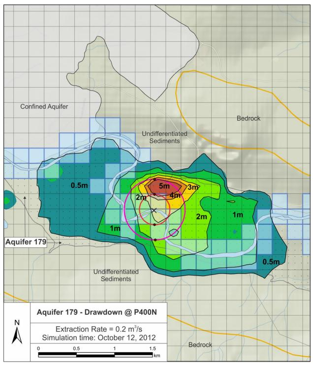
Figure A2.2. Drawdown during distance - sensitivity test. Pumping occurring at P400N location (0.2 m<sup>3</sup>/s).
