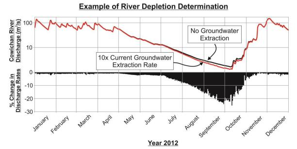
Figure 3.18. Example of the method used for estimating river depletion from pumping an individual well. Shown are the results for RN4 (Marine Harvest Hatchery) in 2012 at 10X current extraction rate.
