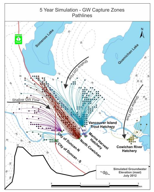
Figure 3.14. 5-year transient groundwater capture zone analysis (2008-2012). Shown are the particle pathlines within the shallow aquifer materials.
