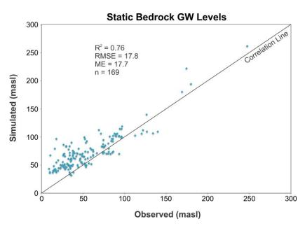
Figure 3.2. Simulated mean annual (2007) bedrock GW elevations verses observed static GW elevations in bedrock from the BC WELLS database.
