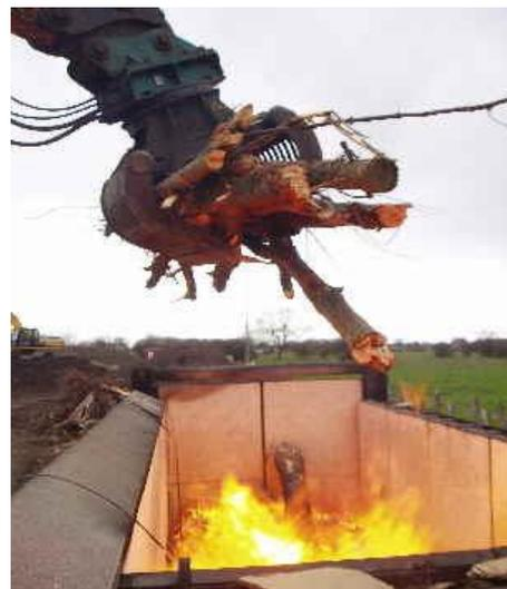
If an air curtain burner is operated properly, there may be slight emissions during start-up and occasionally during feeding as material breaks the curtain of air. However, for the majority of the time, if the material is kept below the curtain of air, and the trench is constructed with deep vertical sides, the result should be a clean, efficient burn.
