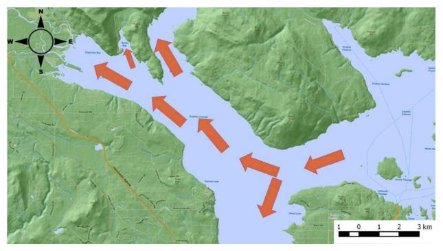
During the ebb tide, two typical scenarios develop. Water flows to the south from Sansum Narrows to Satellite Channel. This southerly flow may encounter northerly flowing water from Saanich Inlet, resulting in eddies near the mouth of Cowichan Bay (Figure 7 and 8). If the water flowing from Saanich Inlet is flowing more to the east, the eddies will not develop and flow at the mouth of Cowichan Bay will be to the south east.
