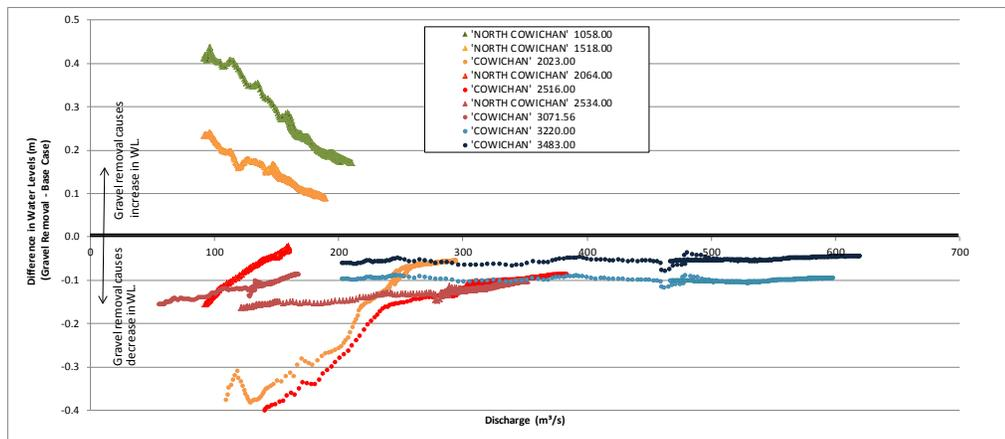
Figure 3: Scenario 1 - Change in water level as a function of discharge.
