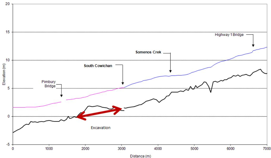
Figure 2: Longitudinal profile of north branch of Cowichan River to Highway 1 Bridge
