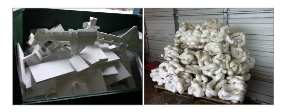
Polystyrene foam before and after processing through the densifier
