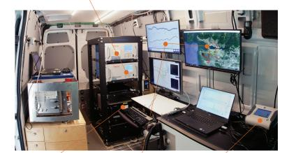
A greenhouse gas analyzer measures carbon dioxide and methane using optical spectroscopy.
