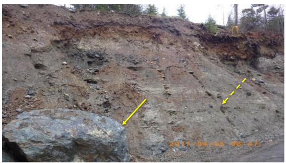
Figure 21. A close up of the glacial till bank. The rock (yellow arrow) can be seen in Figure 22. Note the erosion of the bank material. This bank will be reshaped to eliminate the steep vertical face, in the late summer of 2017. The dashed arrow identifies an erosion rivulet seen in an oblique angle in Figure 22.
